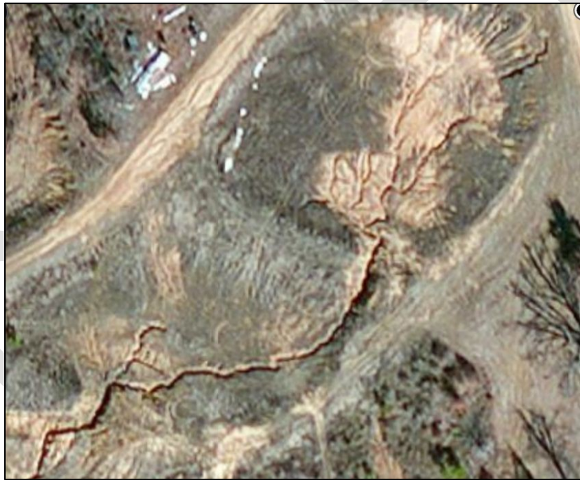
Figure 17b: Typical Gully Sediment Sources: Construction Site
