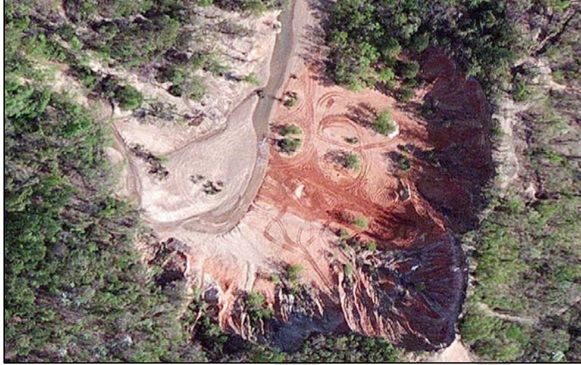
Figure 17a: Typical Gully Sediment Sources: Larger Stream Cut-Bank
