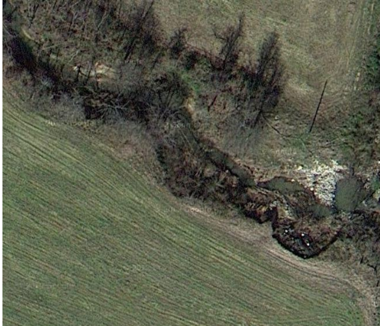
Figure 17c: Typical Gully Sediment Sources: Incising Pasture Creek
