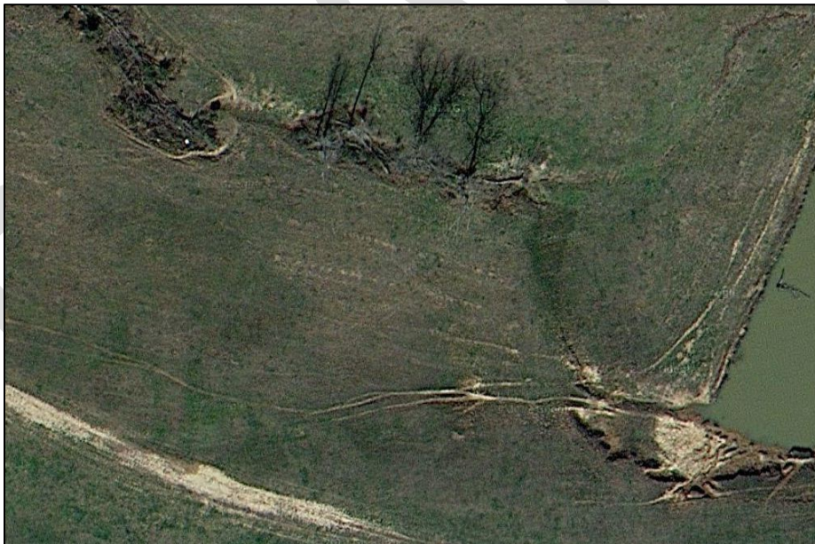
Figure 17d: Typical Gully Sediment Sources: Farm Pond Outlet
