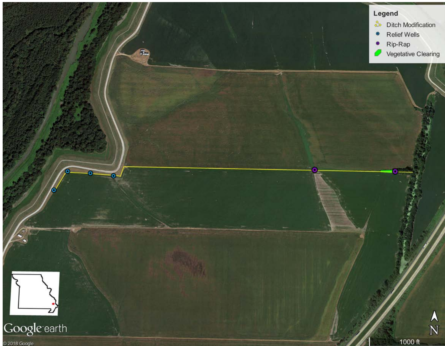
Figure 4. Proposed seepage control measures along the Mississippi River mainline levee at the Below Charleston Mile 24 project area, Mississippi County, Missouri.
