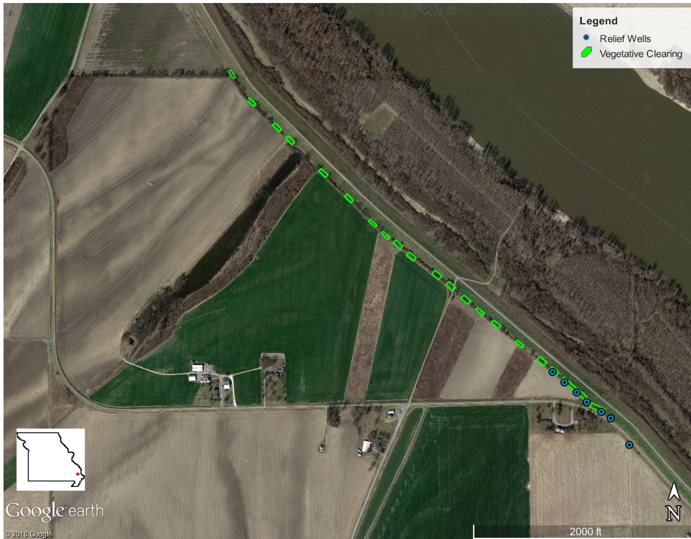
Figure 3. Proposed seepage control measures along the Mississippi River mainline levee at the Below Commerce Mile 15 project area, Scott County, Missouri.
