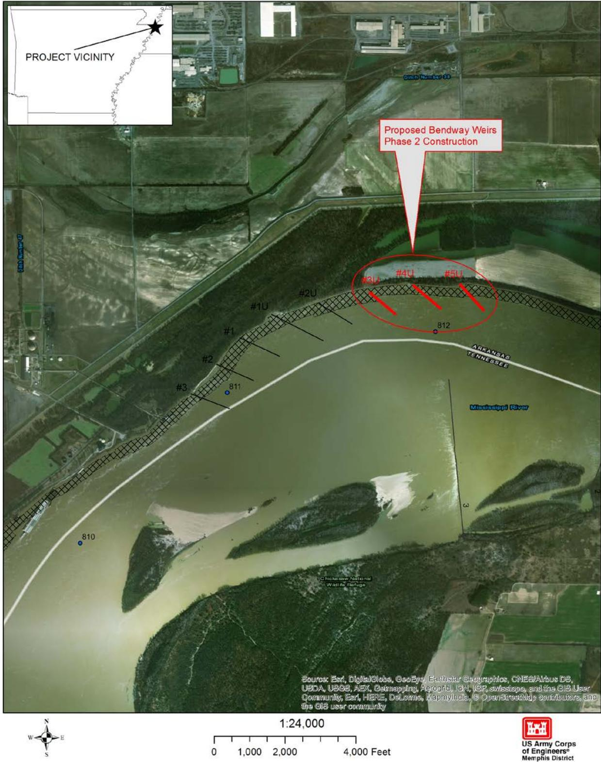
Figure 1. Project map of the three proposed bendway weirs included in Phase 2 construction located along the right descending bank of the Mississippi River near River Mile 812 above head of passes (AHP) in Mississippi County, Arkansas.
