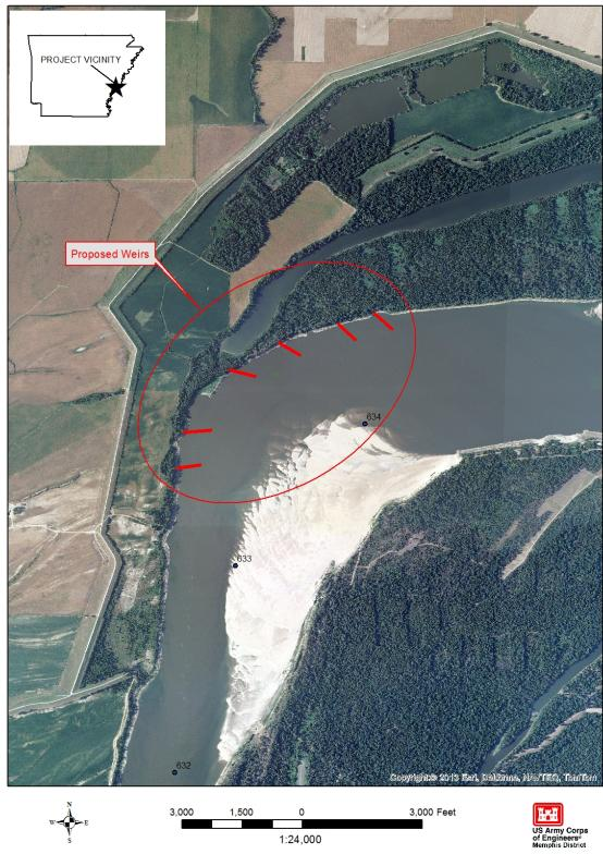
Figure 1. Project map of the six proposed bendway weirs located along the right descending bank of the Mississippi River near River Mile 634 above head of passes (AHP) in Phillips County, Arkansas.
