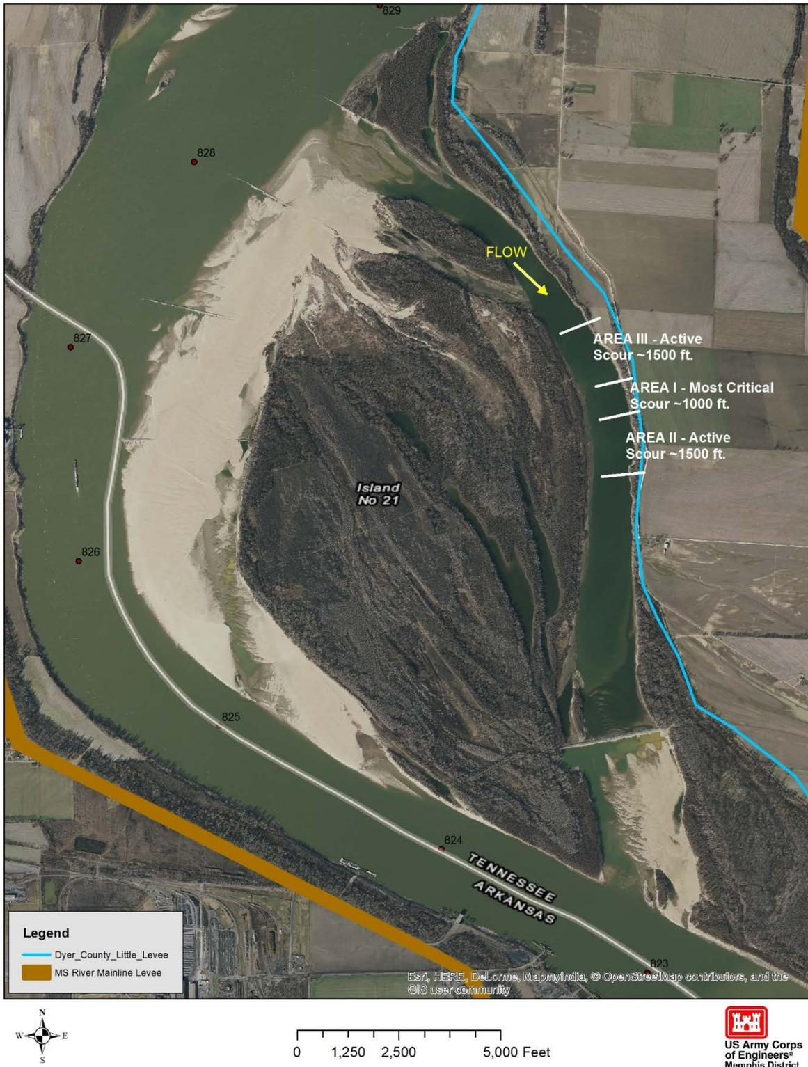
Figure 3. Location of the scour and associated levee rehabilitation measures for the Dyer County Little Levee PL 84-99 Project in northwestern Tennessee.
