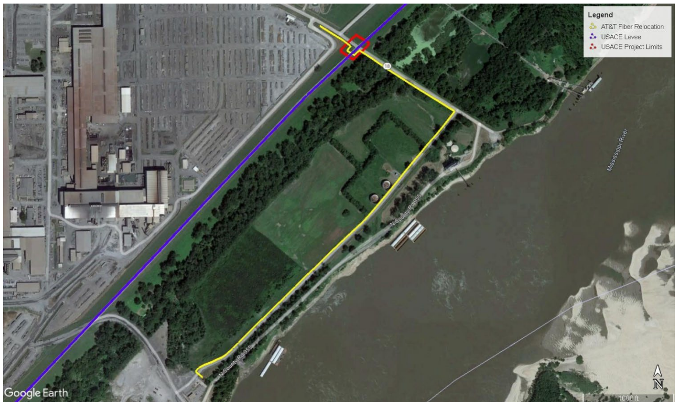
Figure 2. Overview of AT&T fiber installation project details. The yellow line is the proposed line installation, the blue line is the USACE levee, and the red square indicates where the project overlaps the USACE levee.
