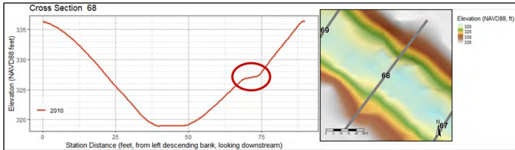
Figure 24. Cross-section 68, illustrating minor left-bank floodplain berm building.
