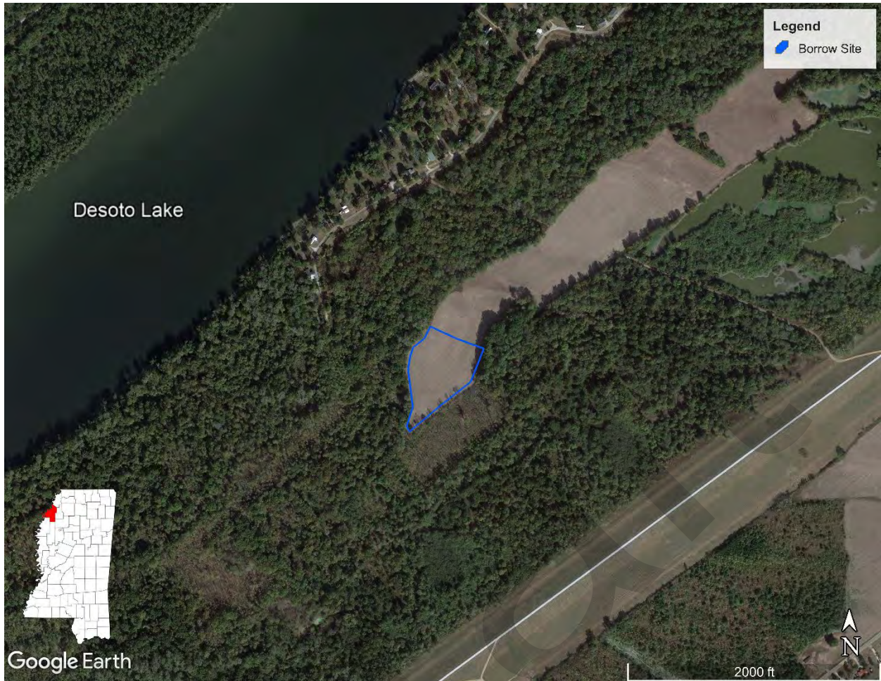
Figure 4. Proposed borrow source location at the Sheard seepage project area, Coahoma County, Mississippi.
