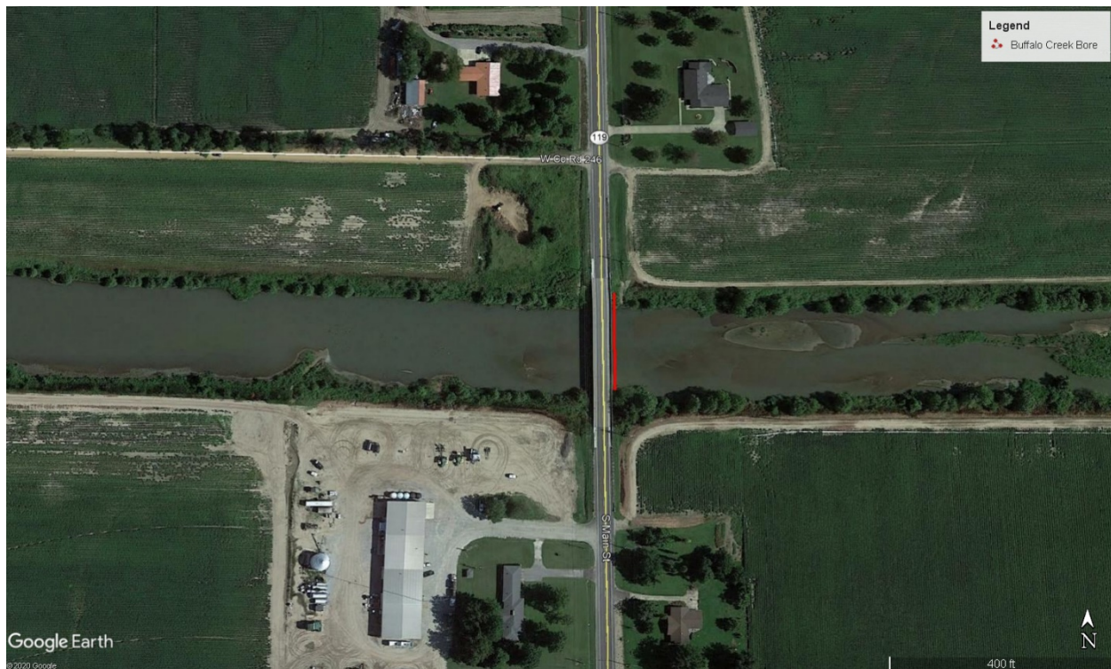
Figure 2. Location of proposed bore to allow tie in of two existing pipes on the north and south side of the bridge.
