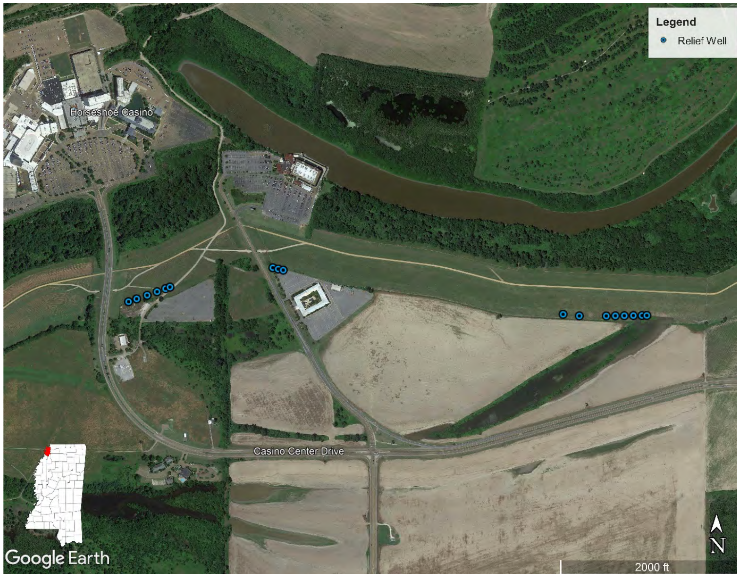
Figure 2. Proposed seepage control measures along the Mississippi River Mainline Levee at the Clack project area, Tunica County, Mississippi.
