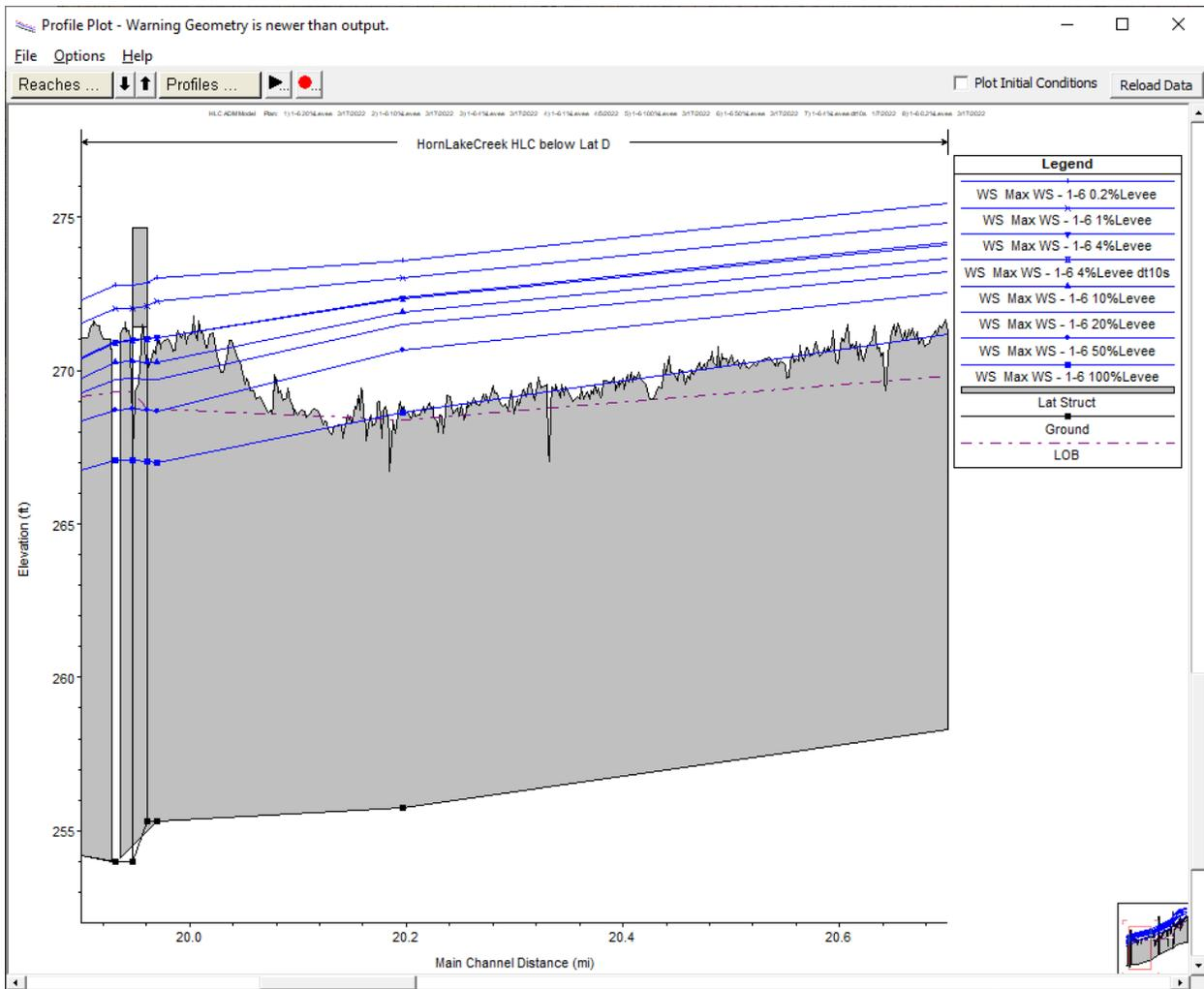
Figure 14. 99.99%, 50%, 20% 10% 4%, 2%, 1%, 0.2% AEP Flood Stages in Horn Lake Creek adjacent to the TSP Levee and Floodwall.
