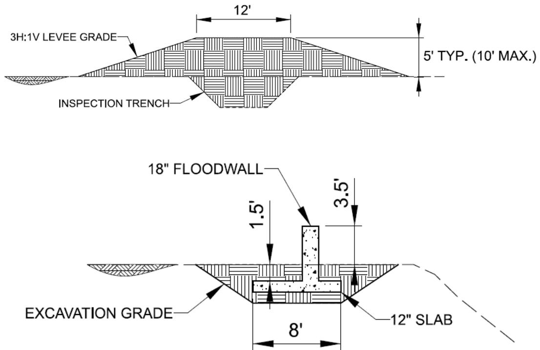
Figure 2: Example Design Cross Section from Plan 8.
