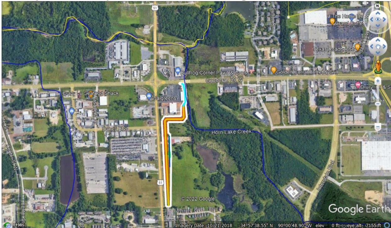
Figure 1: Plan 8 Levee Floodwall Alignment, DeSoto County, Mississippi. Yellow feature is levee and the turquoise feature is the floodwall. Horn Lake Creek flows from Southeast to the Northwest across Goodman Road and Hwy. 51.
