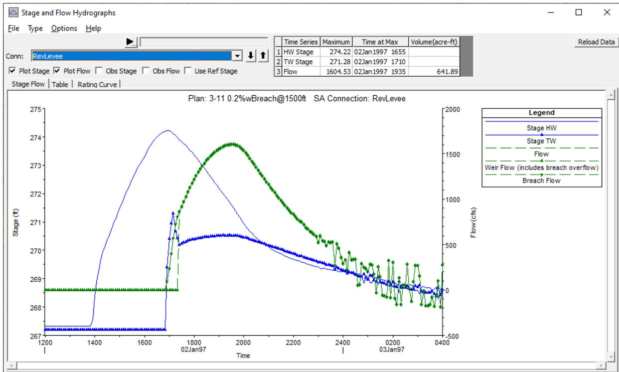
Figure 15. Hydrograph for the 0.2% (500-year) flood at station 15+00 along the levee alignment.
