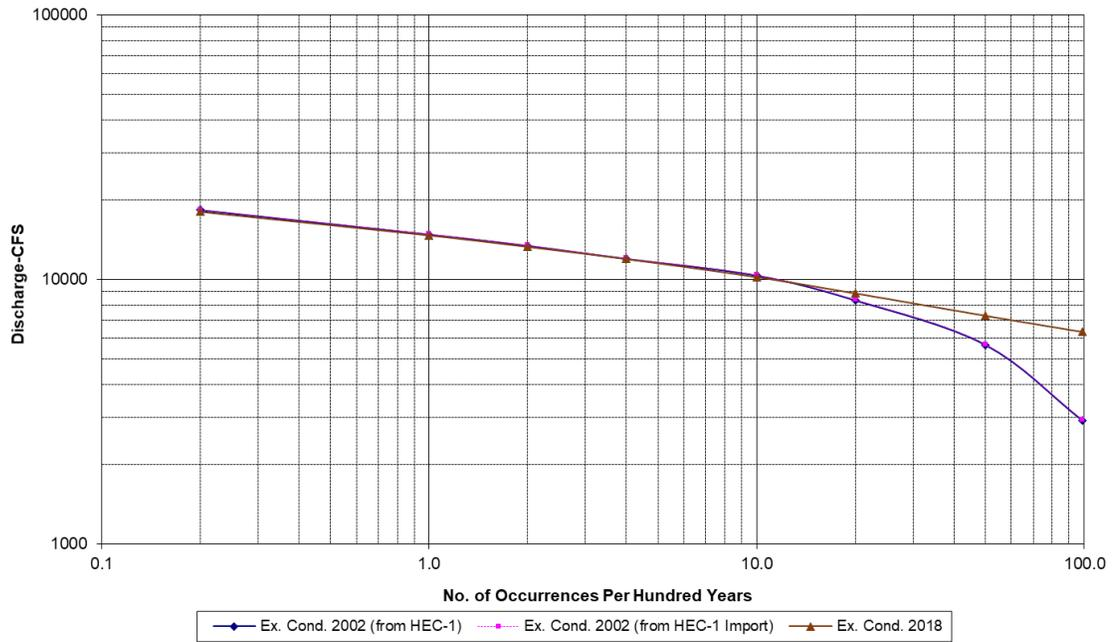
Figure 16. Horn Lake Creek HEC-1 to HEC-HMS Comparison (DA=24.45 Sq.Mi.)
