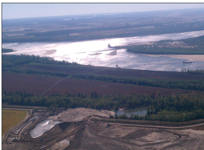
The center crevasse scour hole as seen from the air Oct. 25. The dredge lowa is visible in the channel at top right. (Photo by Brad Hahn, courtesy of Great Lakes Dredge & Dock Company)
