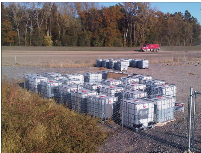
Desensitized blasting agent awaits transport at the upper crevasse. The material will be transported to a disposal site in Illinois.
