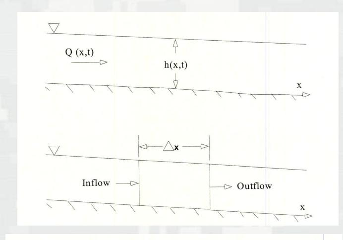
$$\rho \frac{\partial A_T}{\partial t} \Delta x = \rho \left[ \left( Q - \frac{\partial Q}{\partial x} \frac{\Delta x}{2} \right) - \left( Q + \frac{\partial Q}{\partial x} \frac{\Delta x}{2} \right) + Q_I \right]$$
