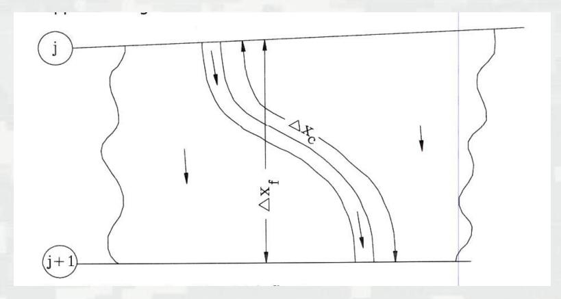
$$\frac{\partial A}{\partial t} + \frac{\partial (\Phi Q)}{\partial x_c} + \frac{\partial [(1 - \Phi)Q]}{\partial x_f} = 0$$
