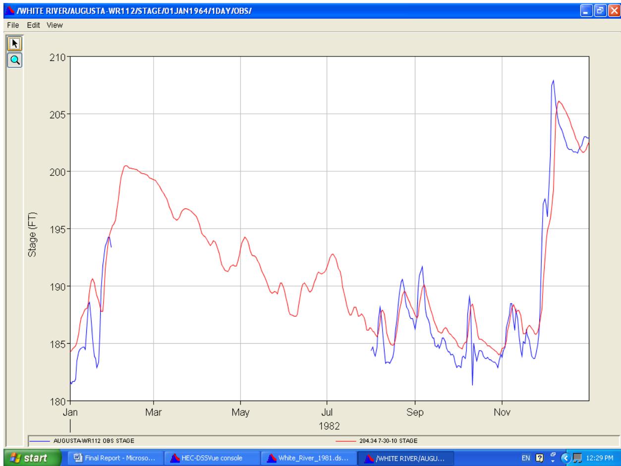
Figure 27. Comparison of 1982 Measured Stages and Unsteady-State Model Results at Augusta
