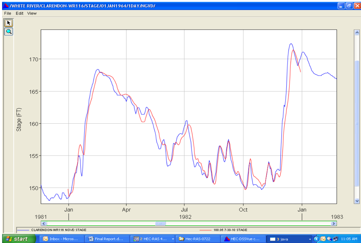
Figure 25. Comparison of 1982 Measured Stages and Unsteady-State Model Results at Clarendon
