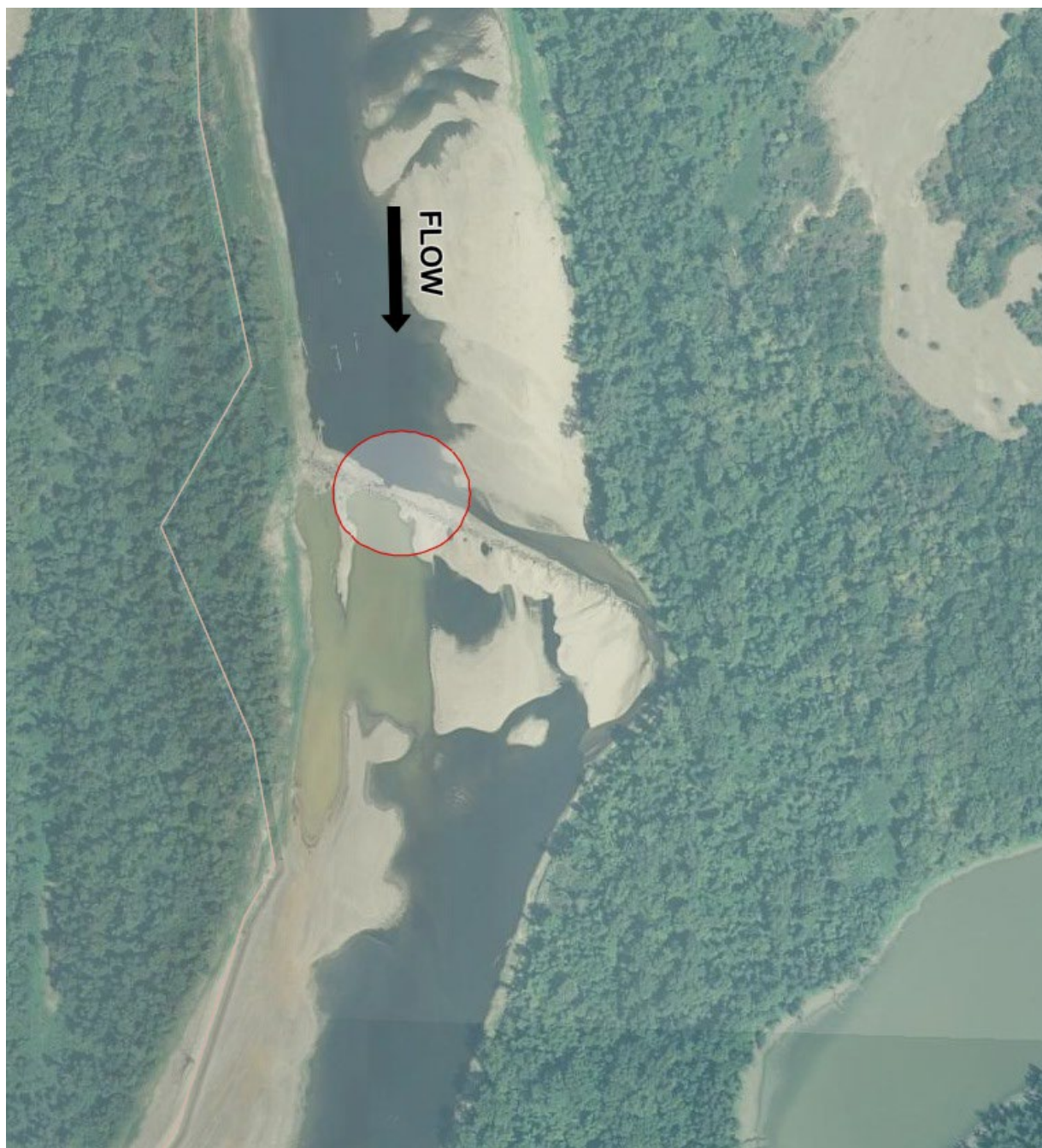
Figure 2-3. Example: Dike Notching Measure to Alter Connectivity (proposed notch shown in red).
