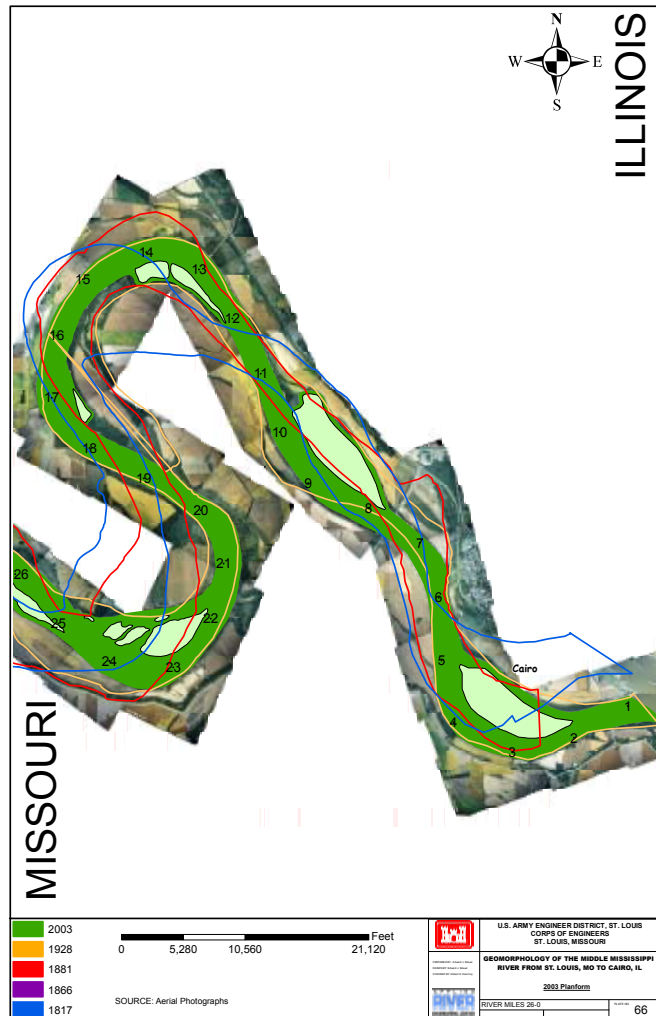
Figure 20. Location of bar and river chute habitats on the Mississippi River in 2003 in relation the channel position from 1812 to 2003 (modified from Brauer et al. 2005).
