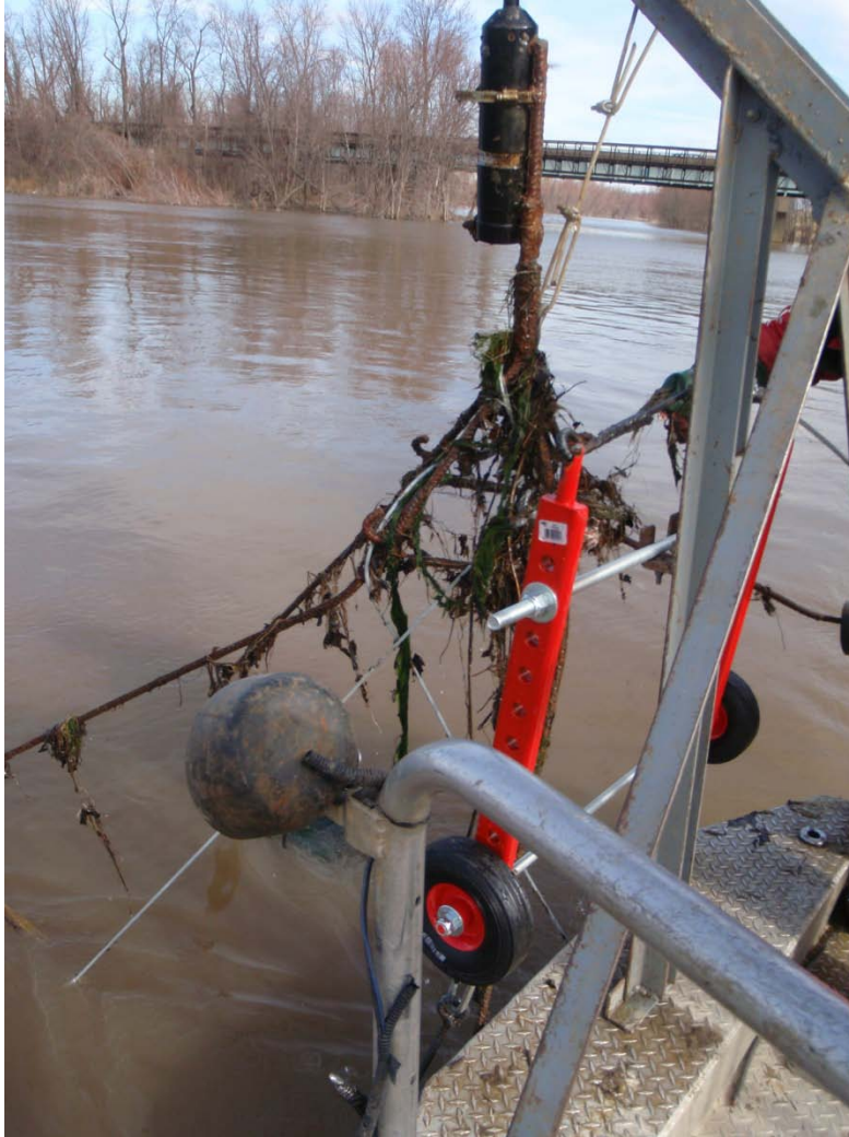
Figure II-3. VR2W on the rebar stand being winched up from the bottom, so that the data can be downloaded.
