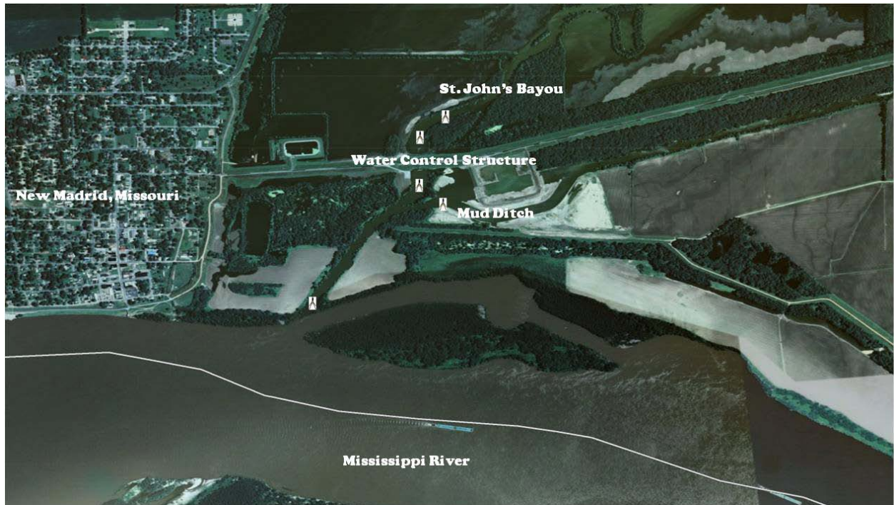
Figure II-1. Locations of VR2W's in St. John's Bayou around the water control structure near New Madrid, Missouri. VR2W locations are shown in the white rectangles.
