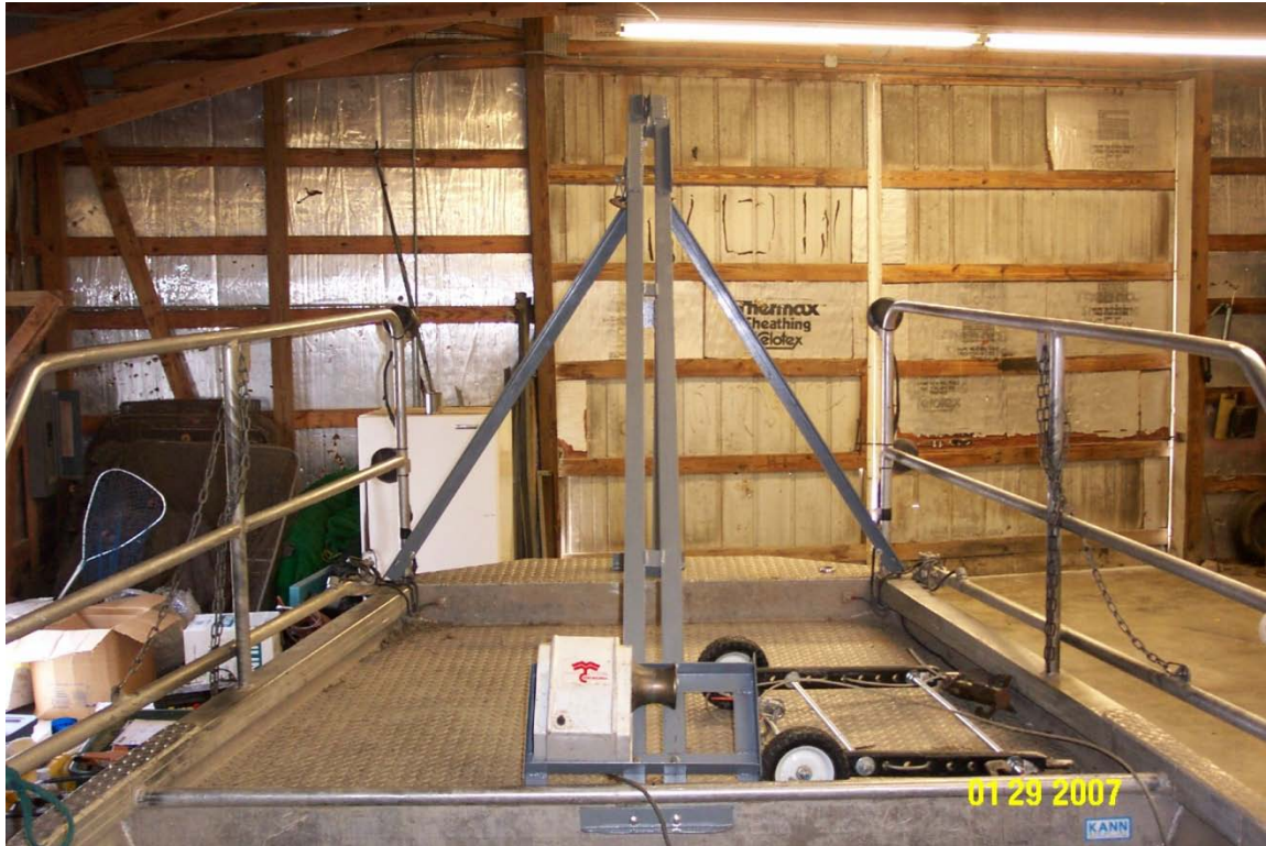
Figure II-2. Boat mounted winch system with grappling contraption of bow of boat that is used to retrieve stationary receivers.
